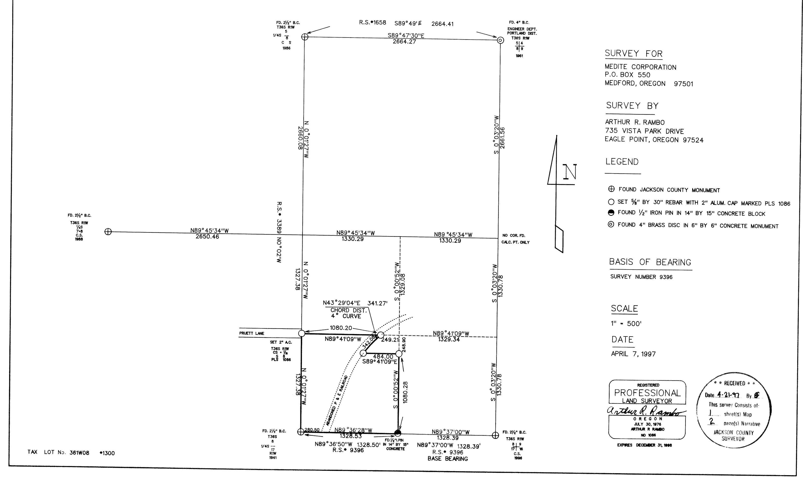
AT THE CENTER SOUTH ONE-SIXTEENTH CORNER SECTION 8, I SET A 5/8 BY 30 INCH IRON PIN WITH A 2 INCH DIAMETER ALUMINUM CAP MARKED:
