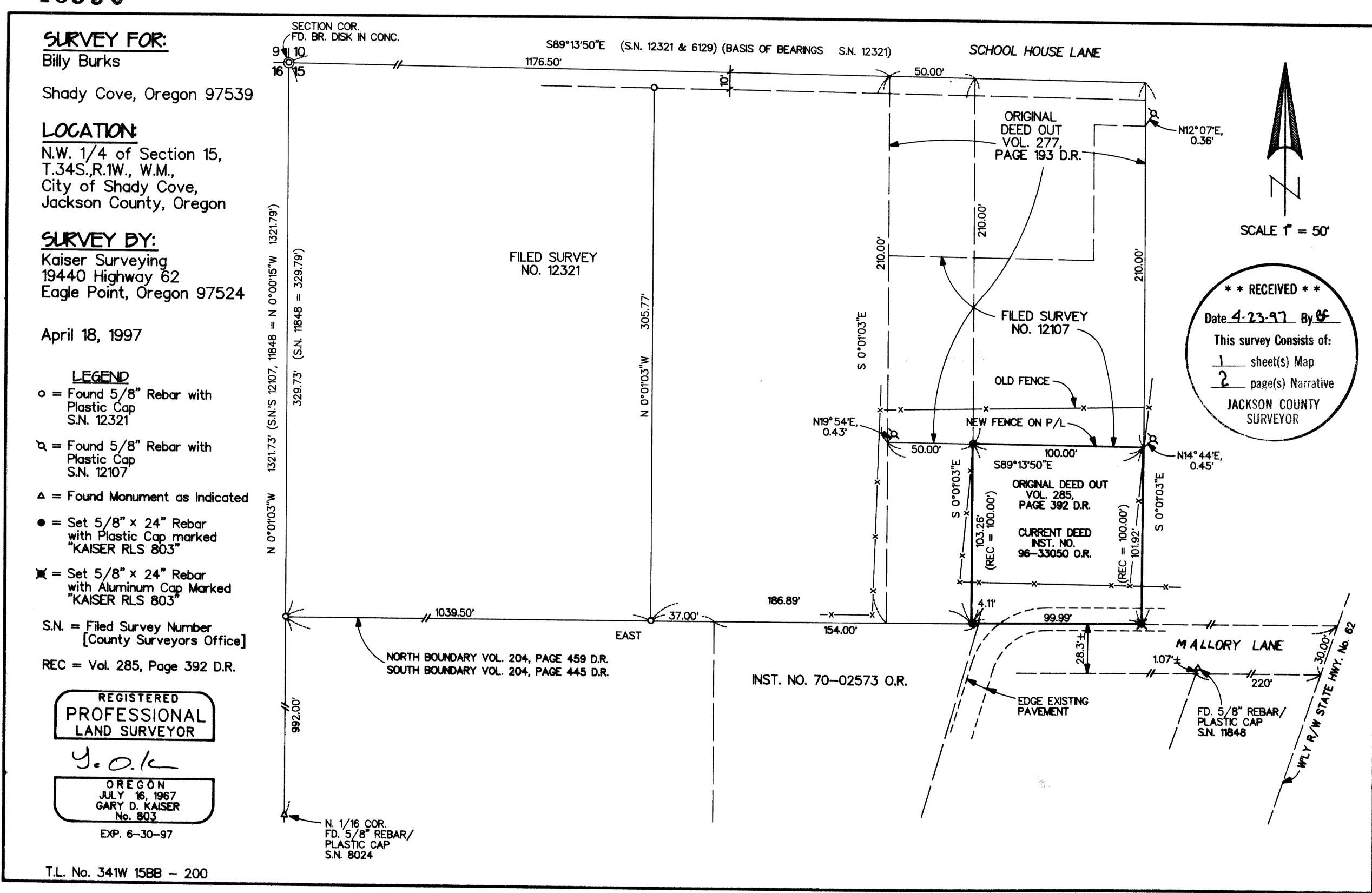
parallel to the North boundary of Section 15 as was also determined by the Surveyor on Filed Survey No. 12107. This left the East and West boundaries of the new Mallory tracts which border on the South boundary of tract described in Vol. 204, page 445, to close on said Vol. 204, page 445, South boundary.
