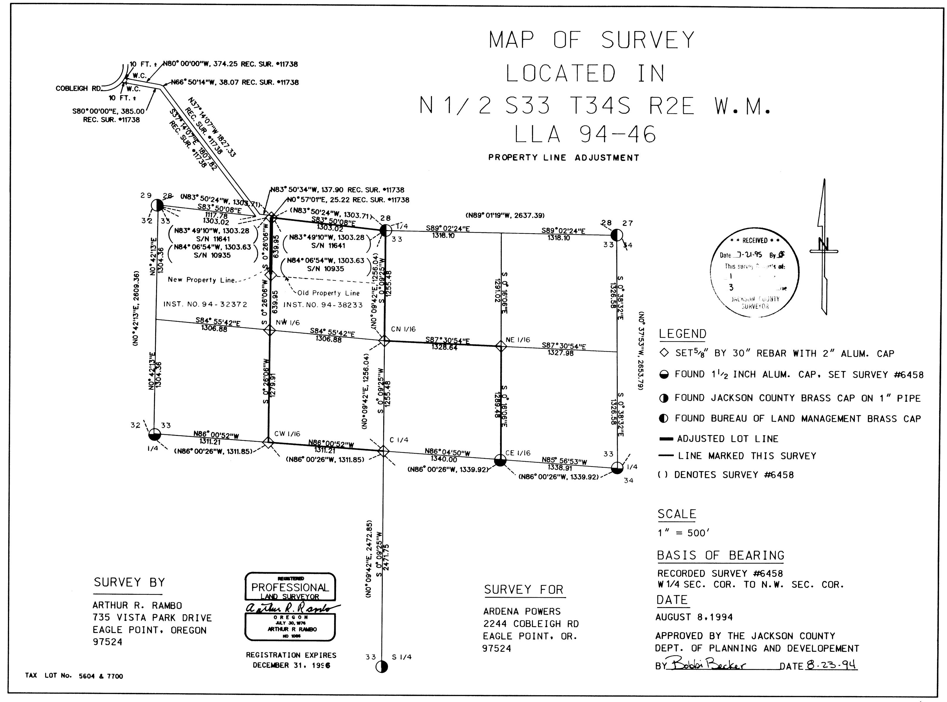
CENTER NORTH ONE-SIXTEENTH CORNER. AT THE CORNER LOCATION I SET A 5/8" BY 30" IRON PIN WITH 2" DIAMETER ALUM. CAP MARKED:
