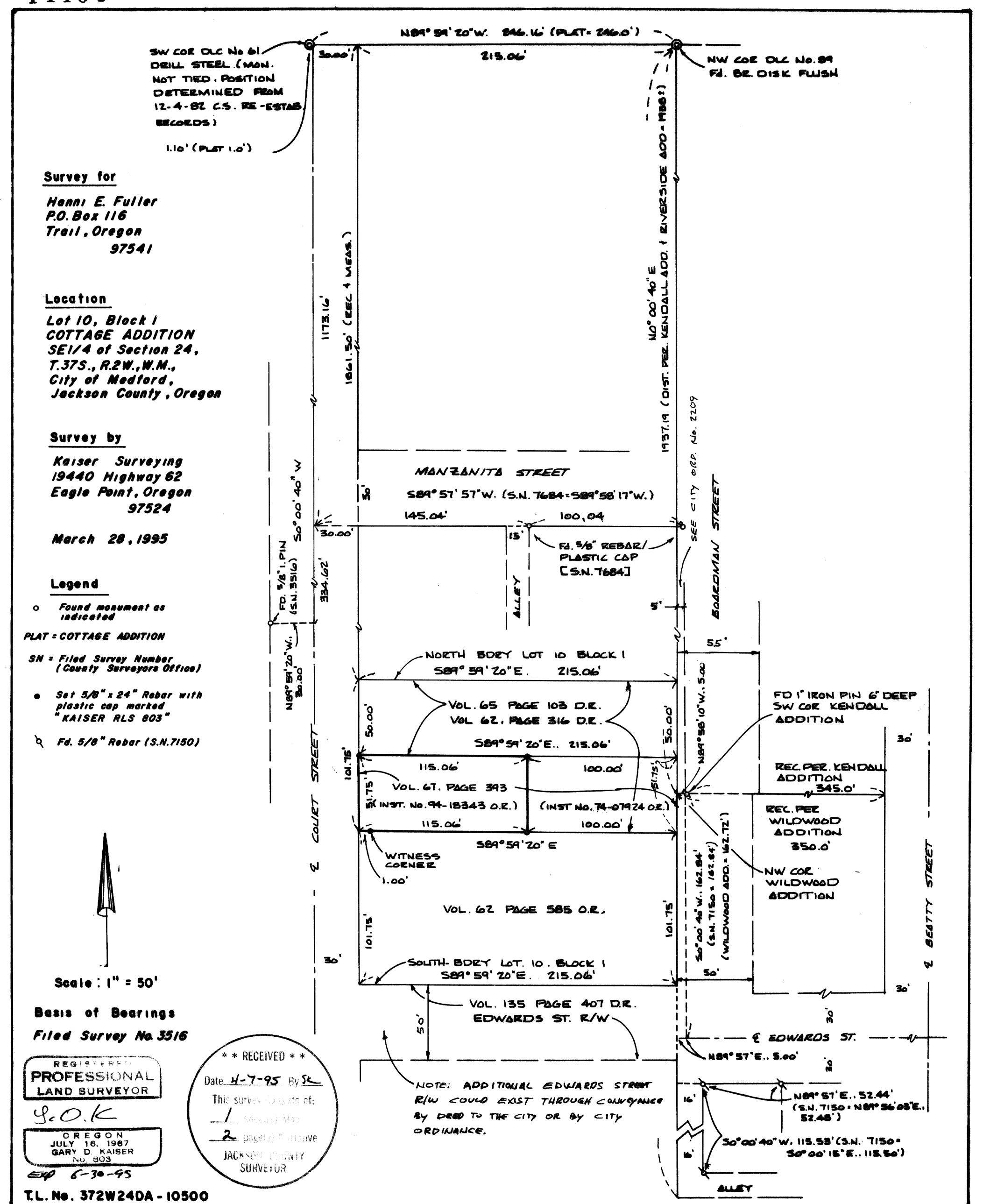
The East boundary of Block 10 was located 5.00 feet West from the 1" iron pin found set for the Southwest corner of Kendall Addition and running North to the NW corner of D.L.C. No. 89. This solution agrees with monuments found set on Filed Survey No. 7150 as shown.
