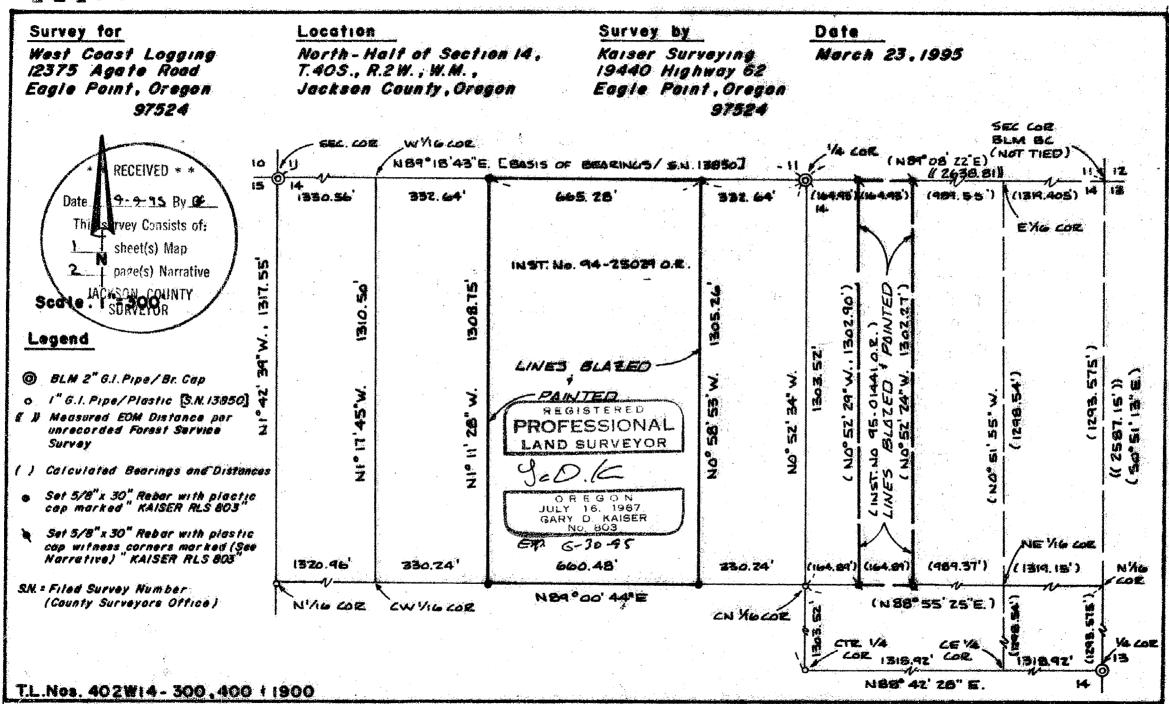
tract were monumented and are to be considered witness corners. Corner positions established by a subdivision of the NE quarter of Section 14 could develop some small differences.
