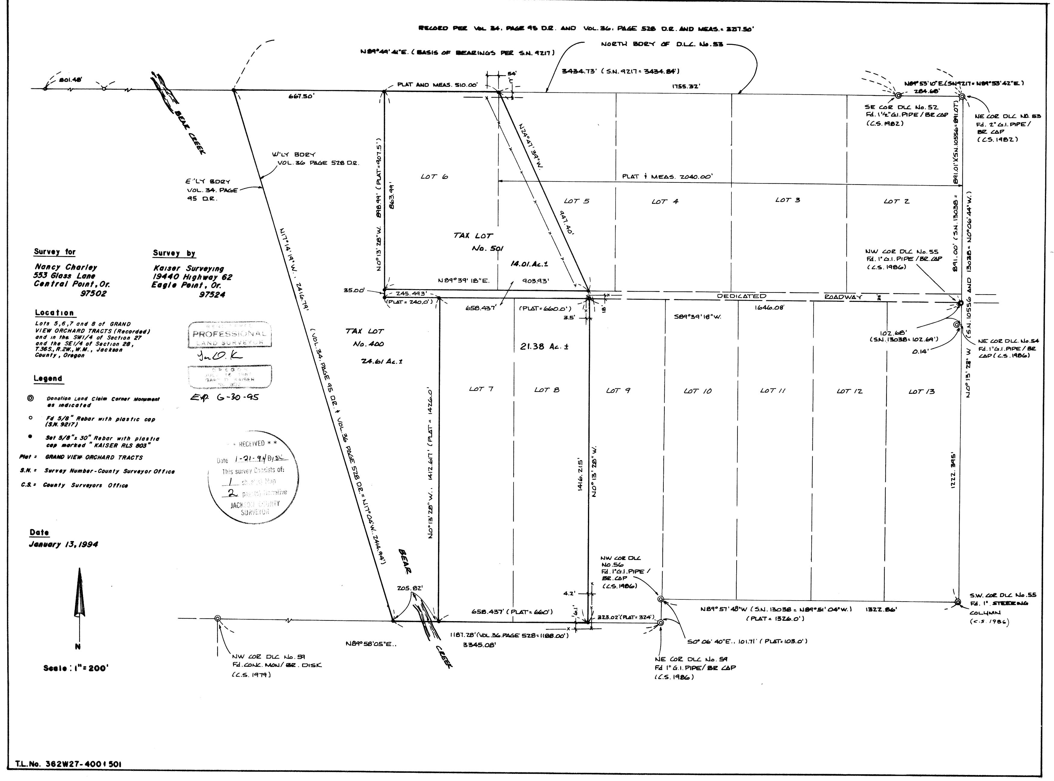
D.L.C. boundary from said intersection point checks the deed record distance to the Northeast corner of D.L.C. No. 59, measure = 1187.28 and Deed Record = 1188.52 feet.
