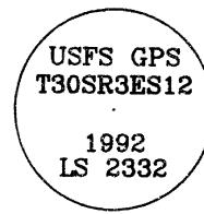
8) A 2-1/2 in. dia. GLO monument, set flush with the ground, improperly marked.
