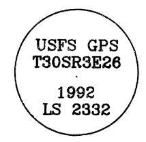
A 5/8 in. dia., 24 in. long iron pin set at the junction of forest roads 6510300 and 6510390, 2 in. below the graveled surface, with a 1-1/2 in. dia. aluminum cap marked:
