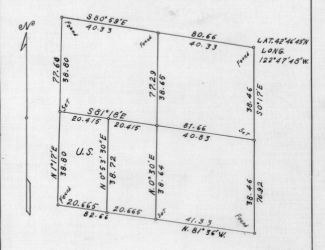
Scale lin = 20 chs = 1320 Ft. The hearings of all lines are referred to the Mean Magnetic Decl. 20°30'E. true meridian determined by solar observations
