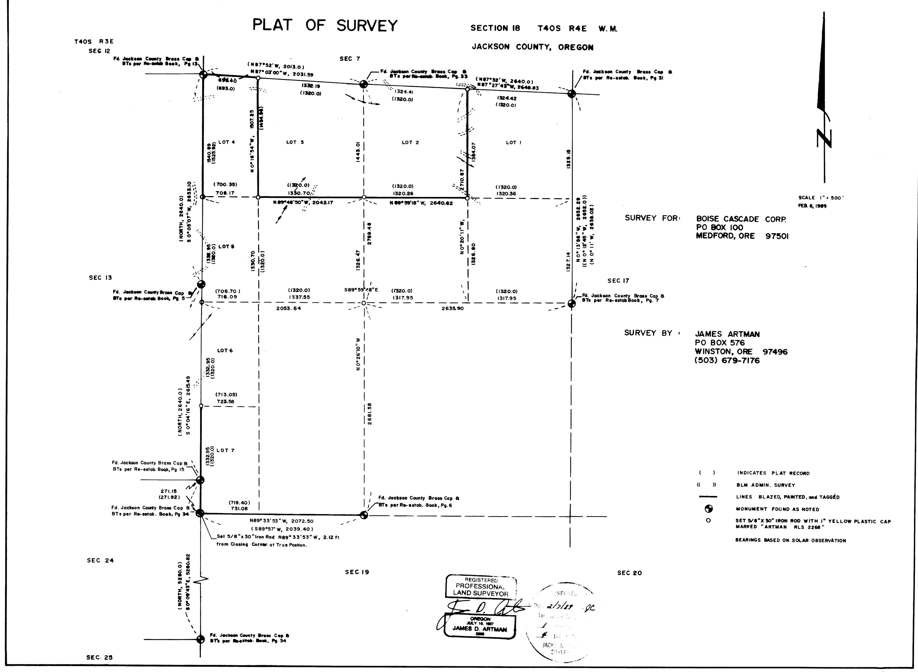
Thence I run on true line N 0°20'11"W, 1384.07 feet to the East 1/16 Corner between Section 7 and Section 18 where I set a 5/8"x30" Iron Rod from which trees bear;
