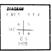
Description of corner evidence found: At the corner point, I found a 2 1/2 inch diameter brass cap monument on a 1 inch diameter iron post protruding 5 inches above ground, marked as shown in the diagram, and the following accessories:
