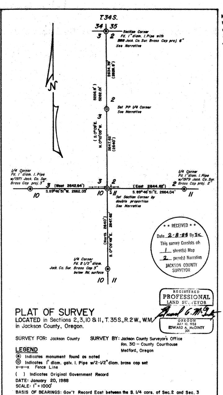
At the quarter corner common to Sections 2 and 3, set a 1x12 ins. galvanized iron pipe  $\frac{1}{2}$  inch below the paving surface of Antioch Road. In the top of said pipe, set in concrete, a  $2\frac{1}{2}$  ins. diam. brass cap mkd:
