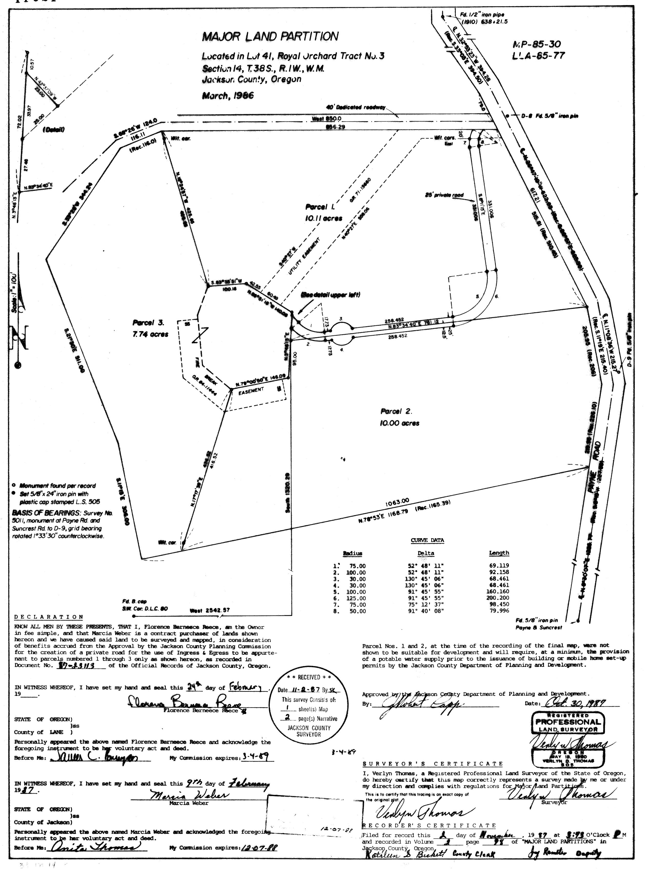
The 1/2" 1910 road pipe at 638 + 21.5, and the 5/8" pin at Payne and Suncrest Roads were held for centerline and intervening tangents between computed on a proportionate basis. 5/8" X 24" iron pins were then set as shown on the accompanying plat.
