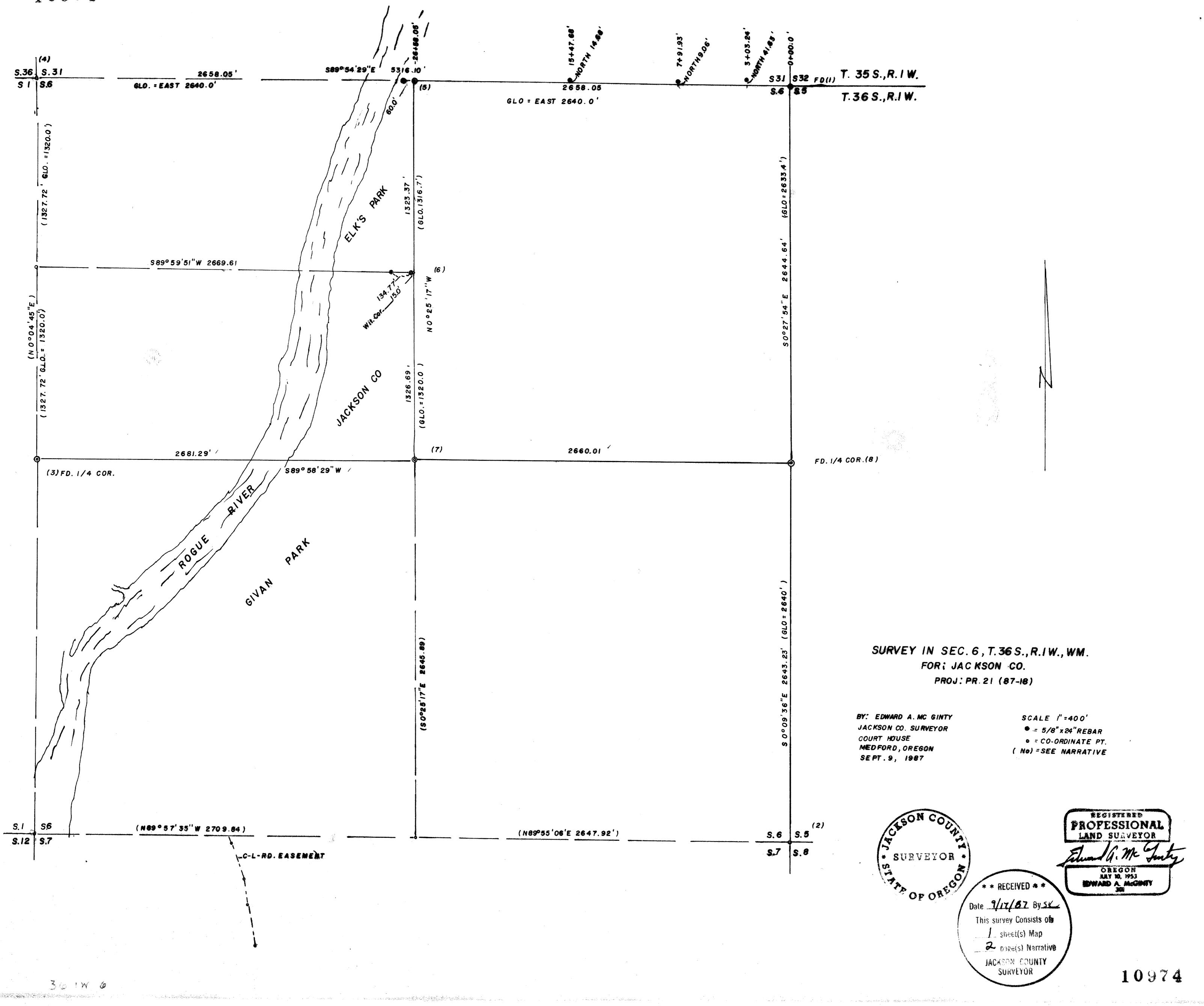
(7) At the center of section, set a 1 inch diam. iron pipe, 36 inches long, flush. This falls approximately 9 feet east of the north-south fence. Osgood monument (lost) computes N23°47'09"W, 17.00 feet.
