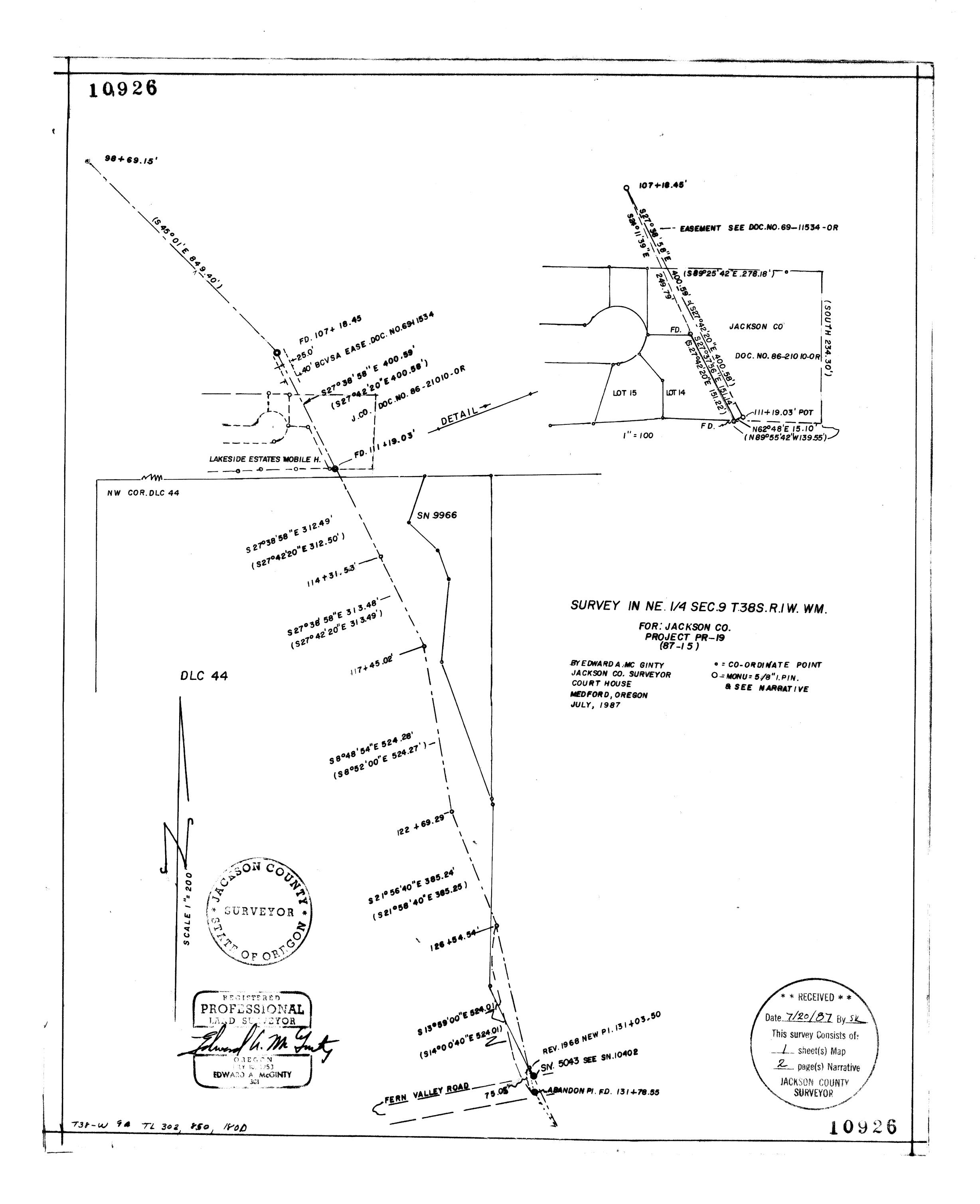
At Station 131+78.55, set approximately 2 ins. deep an iron pin. 5/8 inches in diameter, 24 ins. long with plastic cap mkd. Jackson C.S. from which;
