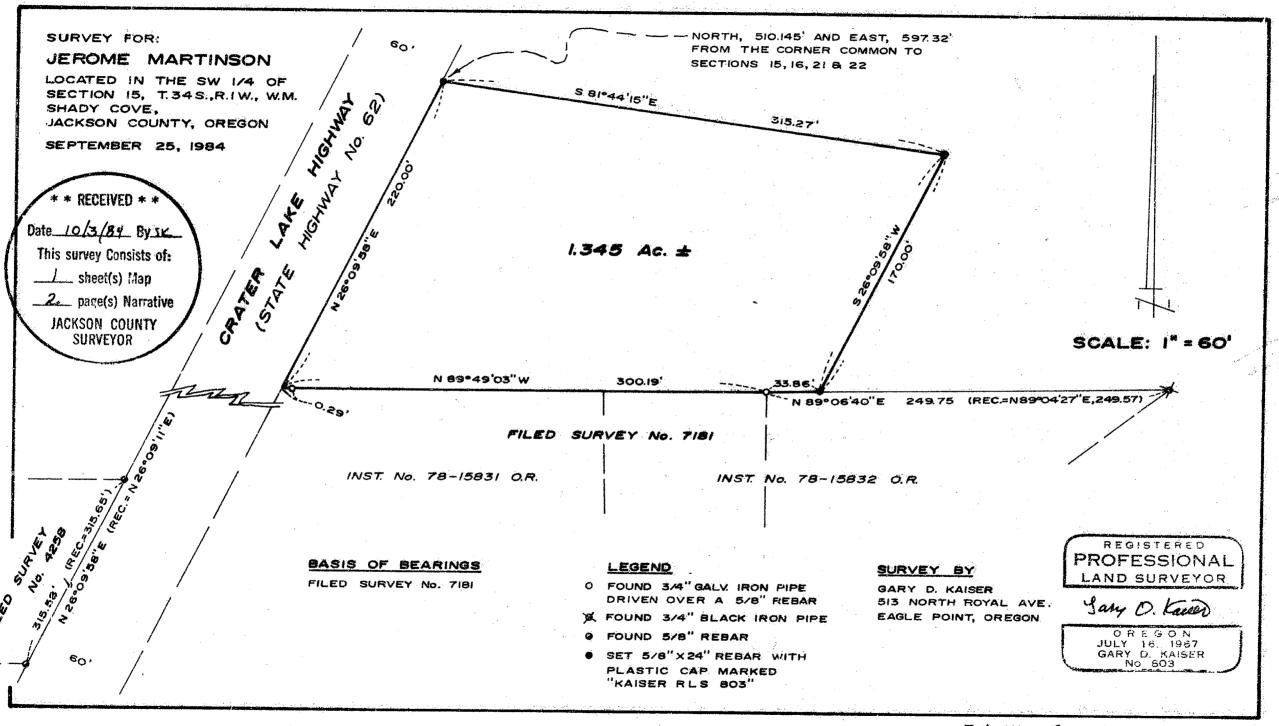
Right-of-way monumentation established on Filed Survey No. 4258 was produced Northeasterly as shown.
