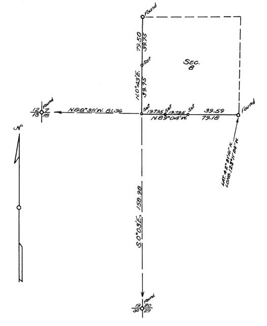
Scale: I in. = 40 chs. = 2640 ft. The bearings of all lines are referred to the true
